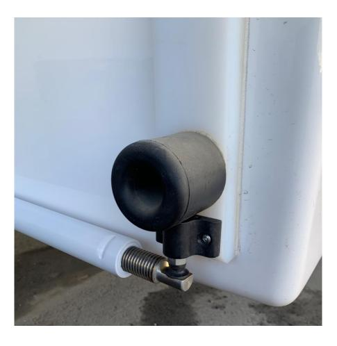
The front mounts are secured with the included hardware into the UHM plastic strip as shown below.
