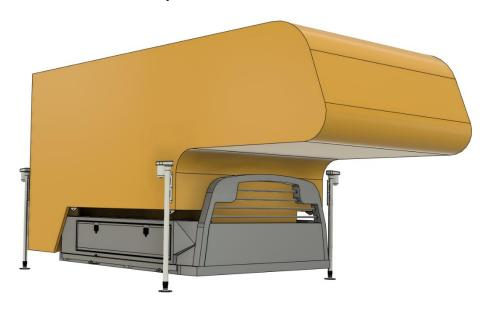
The order of operations for installation of the StableCamper bed kit should start with the Back Stop, and then followed by the Truck Boxes. Stake Pocket Mounts can be installed at any point in the process.
