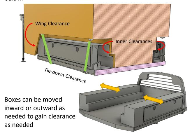
3/8" grade 8 fasteners are supplied for each box. Fastening the boxes to the bed should look like the following image. Care must be taken to ensure hardware locations have clearance under the bed.
